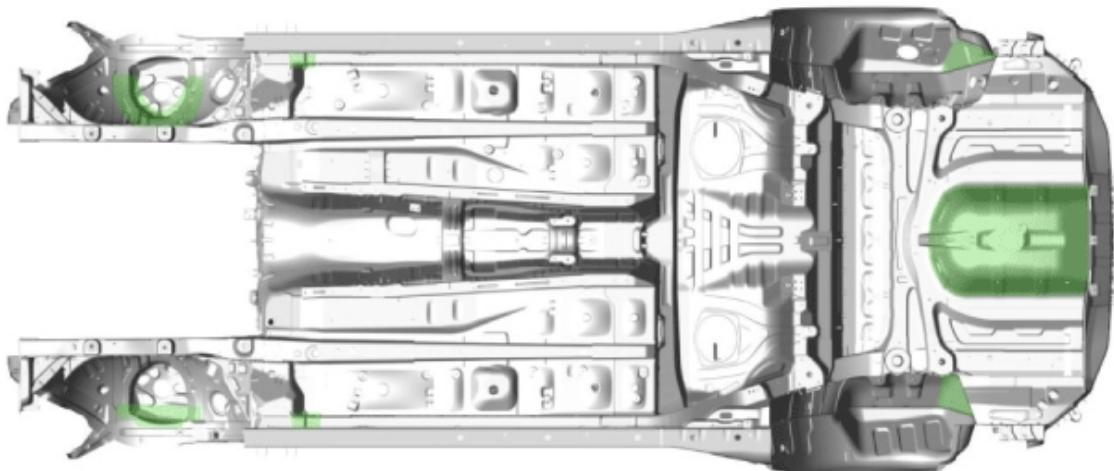
Under body coating (Thickness : 1.0 mm)
